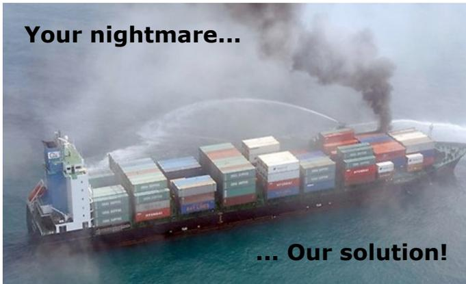
The **OFFMAIN Water Mist Lance** offers superior results if it comes to container fire fighting on board. Specially, when the fire is difficult to access. It **complies** fully with the **IMO regulation** for Water Mist Lance for containerships. This is an easy way to get Water Mist inside a container without opening it. Fast response and efficient extinguishing with small droplets and low water consumption is a winning concept for this type of operation.
